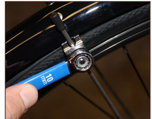
Fig. 12: Rear fender stay adjustment
