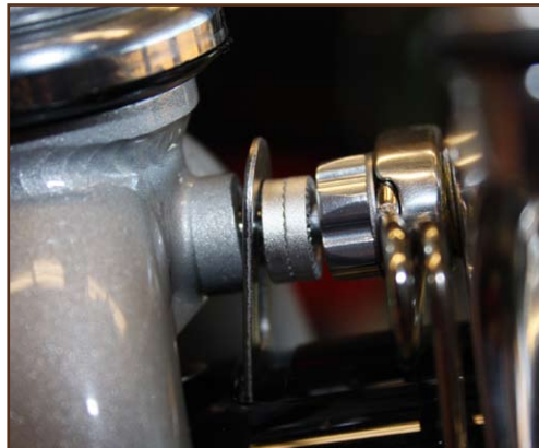
Fig. 3: Front fender L-bracket installation (for road brakes)
