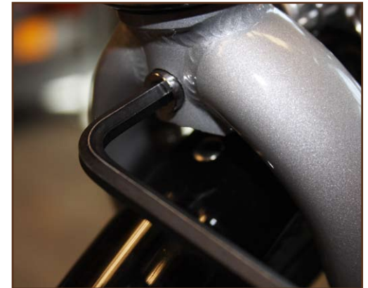
Fig. 4: Front fender L-bracket installation (for road brakes)
