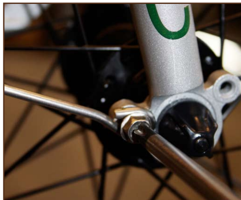
Fig. 5: Front fender stay attachment
