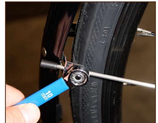
Fig. 6: Fender stay adjustment
